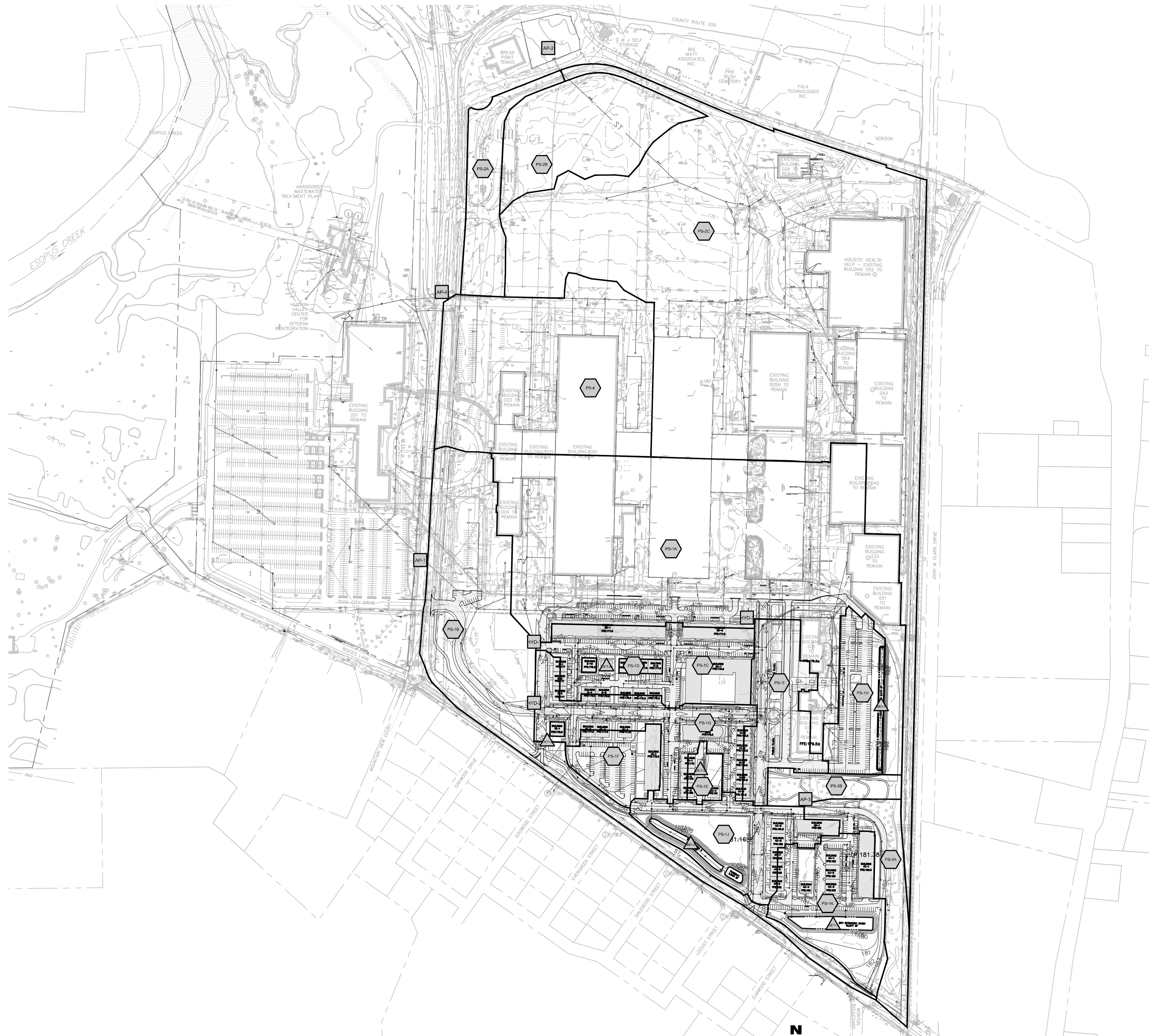
1 POST-DEVELOPMENT WATERSHED DELINEATION MAP FIG. A-7 SCALE: 1" = 200'
